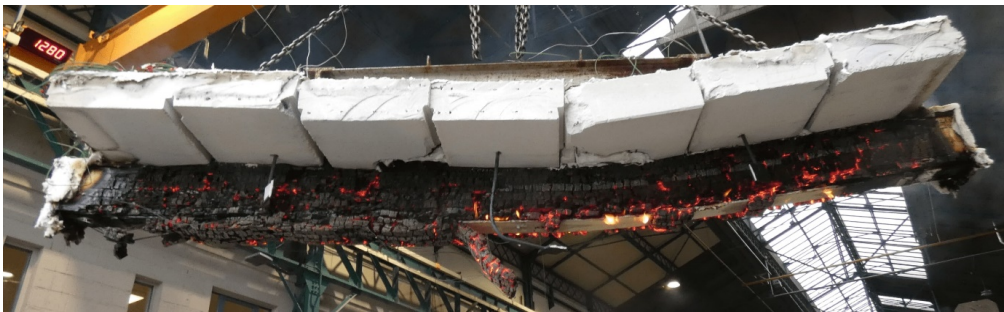
Figure 5: Picture of STC2 beam after being extracted from the furnace
