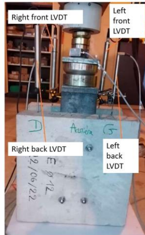
FIGURE 2. Experimental set-up of the pushout test performed to characterize connection behavior (the positions of the four LVDT sensors used as well as the vertical jack and the pancake load sensor used are shown)
